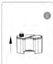
Put the water tank base up.
