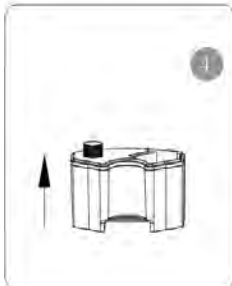
Put the water tank base up.
