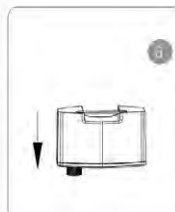
Screw tank cover tightly and put it in to the fan, then close the panel.
